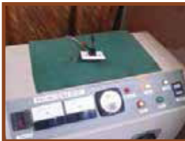
Switch - high voltage test
